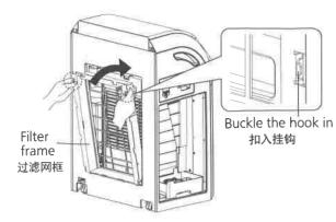
(10)Install the pre-filter, with the handle outside. 将带把手面朝外,安装预过滤网。
