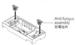
(3) Push the mist holder to the right for unfixing, then put down and buckled the hooks in.
