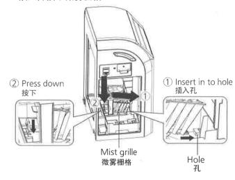
(6)Install humidifying filter cap with the handle outside. 带把手面朝外, 安装加湿过滤网压板。
