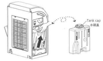
(3)Unscrew tank caps and fill the 2 tanks with water。 拧开水箱盖并给2个水箱加水。
