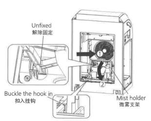
(5)Install humidifying filter. (There is no distinction between sides.) 安装加湿过滤网。(没有内外的区分)
