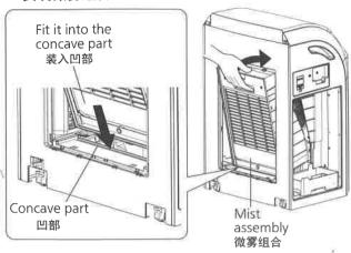
(9)Install the HEPA composite filter, with the black side outside.
