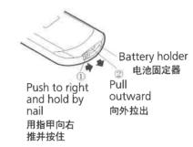
② Install battery with ⊕ facing up into battery holder. 将电池①向上放入电池固定器。
