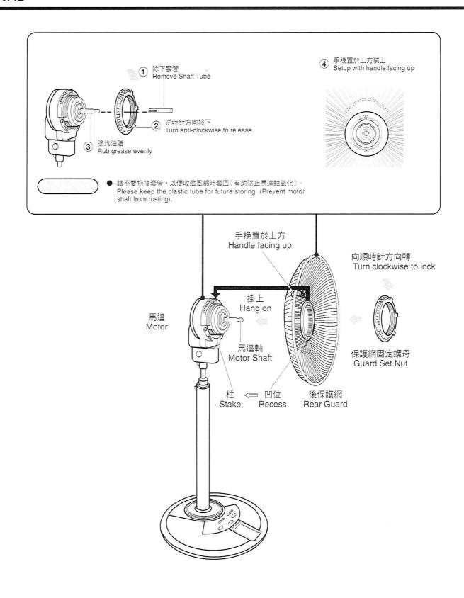
● 請確保擰緊保護網固定螺母和旋蓋以防在使用中鬆脫。 Please tighten the guard set nut and spinner firmly to prevent them from loosening.
