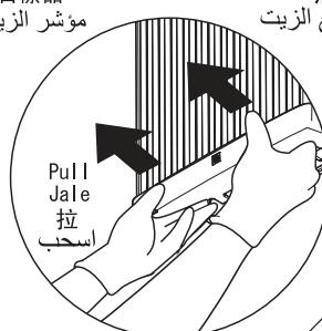
Hold knobs and pull the oil cup like picture.
