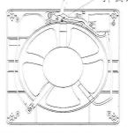
7 Secure the orifice with four screws (Make sure the orifice don't crimp any elcectrical wires). Then attach the louver (Push the louver until it clicks and secure it with the two screws).
